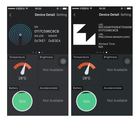
The Sensoro app supports setup of beacon's basic information (including UUID, Major and Minor) as well as the modification of device transmitting power, radio frequency, and other parameters.
